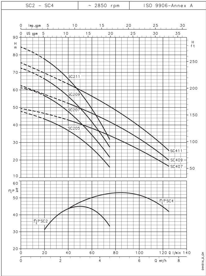
These performances are valid for liquids with density  $\rho=1.0~kg/dm^3$  and kinematic viscosity  $\gamma=1~mm^2/sec$ .
